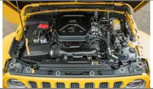
3. Remove (3) three, 10mm bolts from the OEM headlight assembly. Repeat on other side.
